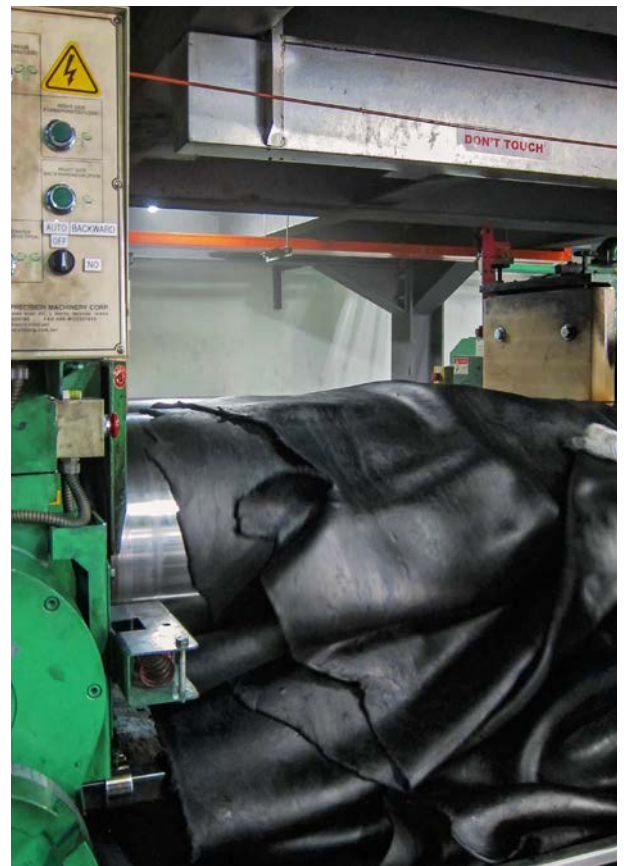
Finalized compound on rolling mill
