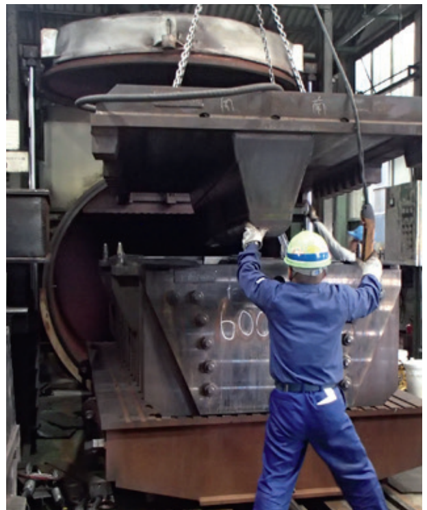
Closing mold with counterpart prior to curing
