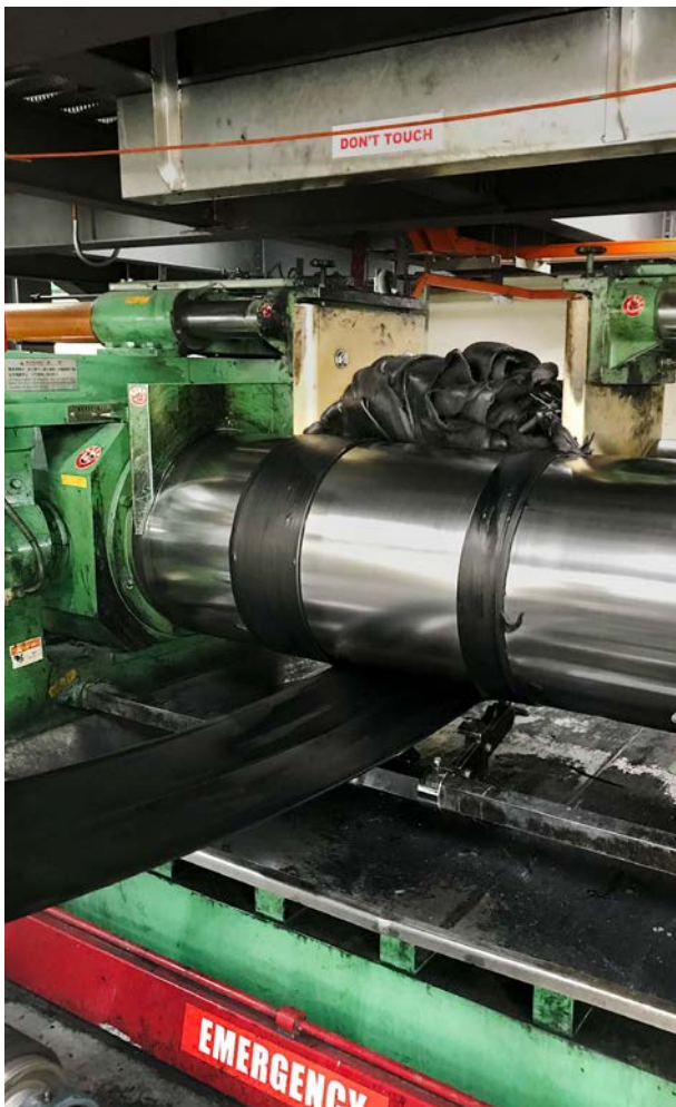
Masterbatch on rolling mill
