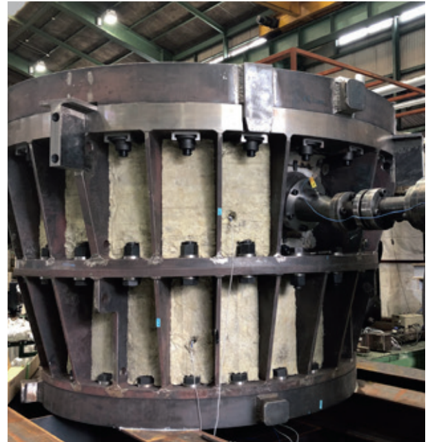
Jacket mold with bolts during high pressure injection of rubber
