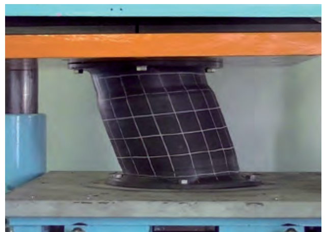
CSS Fender shear testing with panel and UHMW-PE face pads
